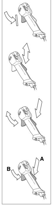
• See section "Start". Start the machine and apply full throttle. Release the throttle and check that the cutting equipment stops and remains at a standstill. If the cutting equipment rotates with the throttle in the idling position then the carburettor's idling setting must be checked. See chapter
